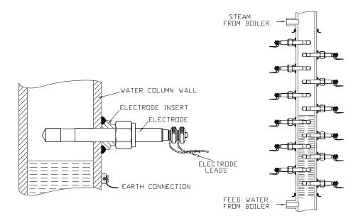
Figure 1.1 - Schematic of high pressure resistance measuring cell and electrodes
